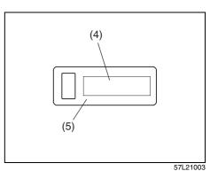
The key identification number (4) is stamped on a metal tag (5) provided with the keys. Keep the tag in a safe place. If you lose your keys, you will need this number to have new keys made. Write the number below for your future reference.
